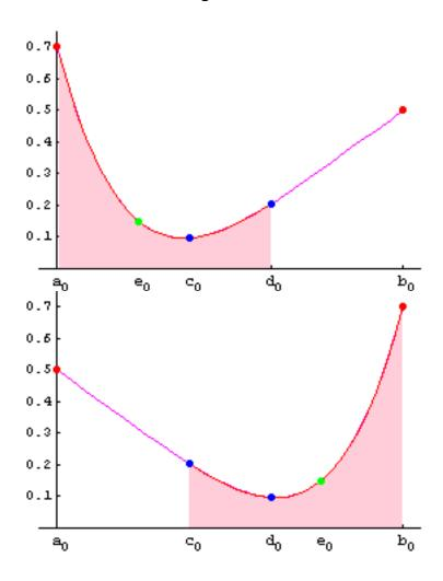
If  $f(c_0) \le f(d_0)$ , then squeeze from the right and left and use the new interval  $[a_1, b_1] = [a_0, d_0]$ .
